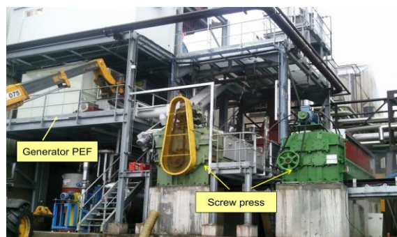
Figure 4: Industrial equipment for PEF treatment installed at the sugar factory.
